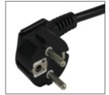
Type: DIN49441 Rating: 16A 250VAC Code: DINM
